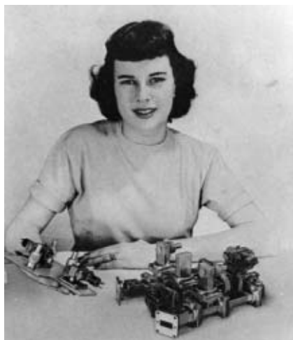
▲ Fig. 3 A comparison of Tri-Plate Modules to waveguide. (Courtesy of Sanders Associates.)
