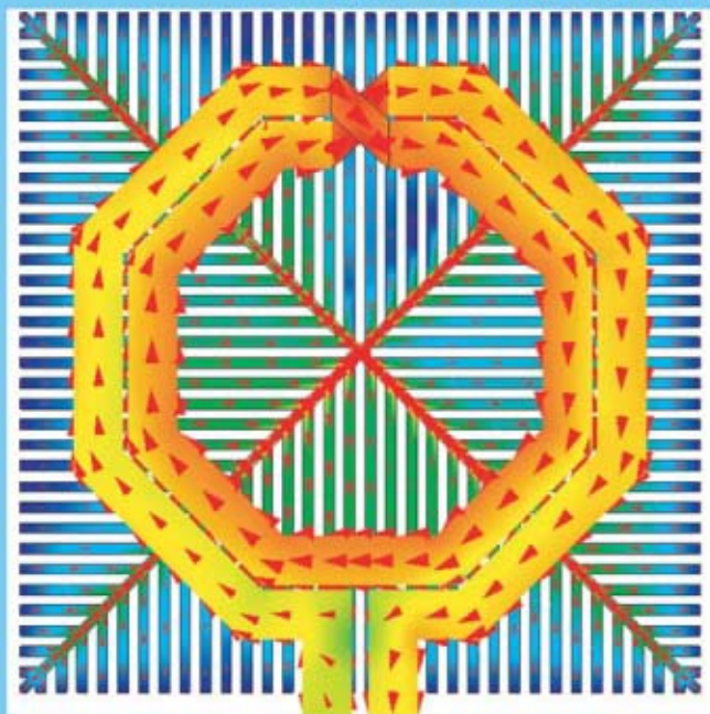
Current Distribution Visualization on a RFIC Cell
