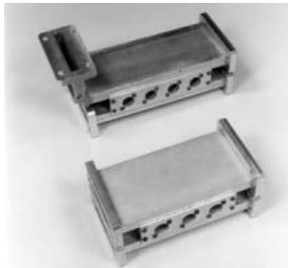
▲ Fig. 5 High power branch arm couplers in \frac{1}{2} height waveguide.
