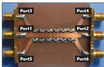
▲ Fig. 8 The six-cell trisecting power divider with a symmetric structure (LH, RH, LH).
