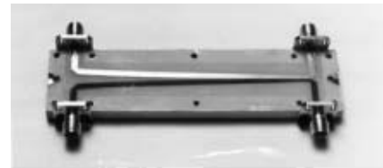
▲ Fig. 6 An asymmetric tapered-line coupler.
