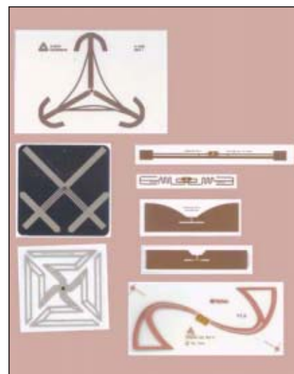
▲ Fig. 2 Examples of UHF passive RFID tags.
